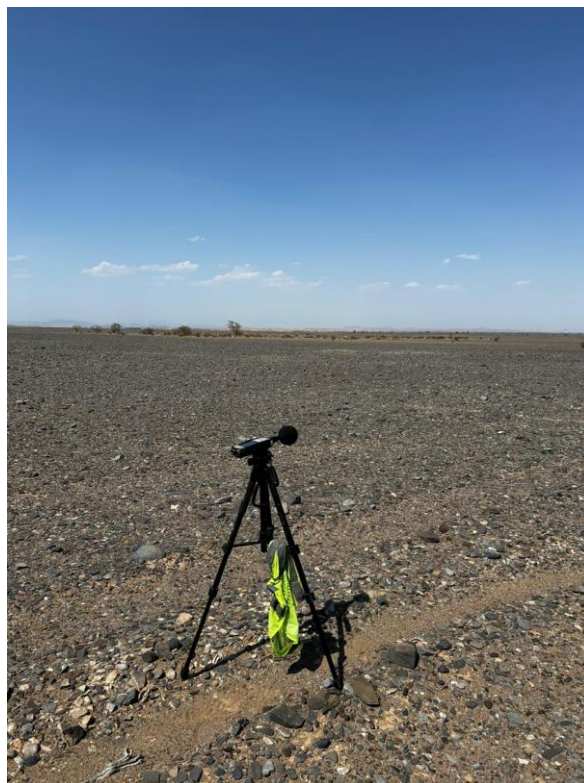
Figure 4-10 Noise Monitoring at Manah I Solar PV undertaken by HMR team on 31 th April 2023
